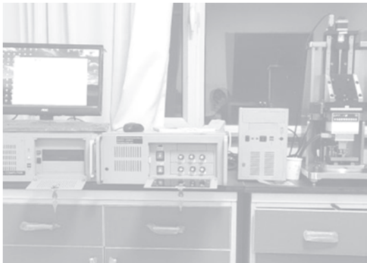
图 1 CFT-I 型常温摩擦磨损试验仪 Fig. 1 CFT-I normal temperature friction and wear tester
