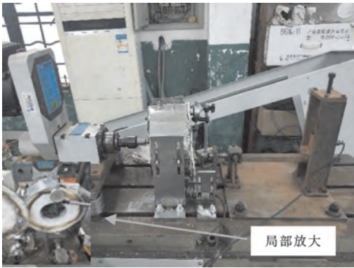
图 5 高温轴承游隙测量实验台 Fig. 5 Test bench for high temperature bearing clearance measurement
