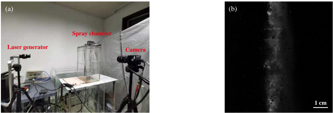
Fig. 3 (a) Physical diagram of PIV measurement system, (b) Mist spray photo under 6.9 MPa 图 3 (a) PIV测量系统实物图, (b) 6.9 MPa下的喷雾照片
