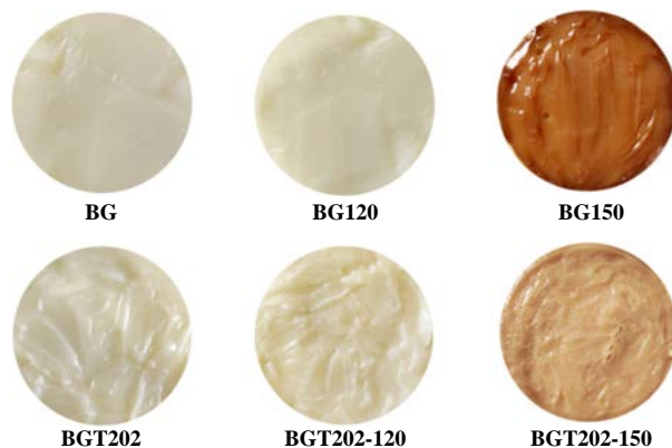
Fig. 1 The appearance of lithium complex greases before and after heated at 120 and 150 ℃ for 24 h
